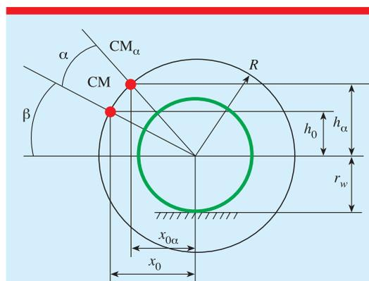
**Figure 4.** The geometry of the change in position of the centre of mass from inclining the bike is seen in this enlargement of the rear wheel. The line connecting the centre of mass of the horizontal bike and the rear wheel makes an angle  $\beta$  with the  $x$ -axis, whereas that of the inclined bike ( $CM_\alpha$ ) makes an angle  $\alpha + \beta$ .  $h_0$  and  $h_\alpha$  are the  $y$ -coordinates of  $CM_0$  and  $CM_\alpha$ , respectively, and  $r_w$  is the wheel radius.
