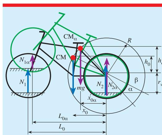
**Figure 2.** Schematic diagram of forces acting on the bike in the horizontal and inclined positions (for clarity the rider is not shown).  $N_1$  and  $N_{1\alpha}$  are the normal forces acting on the front wheel for the horizontal and inclined states, respectively, and  $N_2$ ,  $N_{2\alpha}$  are those for the rear wheel. CM and  $CM_\alpha$  are the locations of the centre of mass for the horizontal and the inclined positions, respectively.
