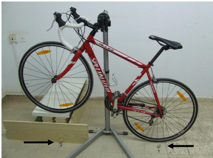
**Figure 3.** Inclined bike. In order to easily measure  $L_{0\alpha}$  we hang small weights from the rear and front hubs, which serve as plumbs (see the arrows). Note that the system configuration is only an approximation for a real slope as the bicycle rests on horizontal slabs.
