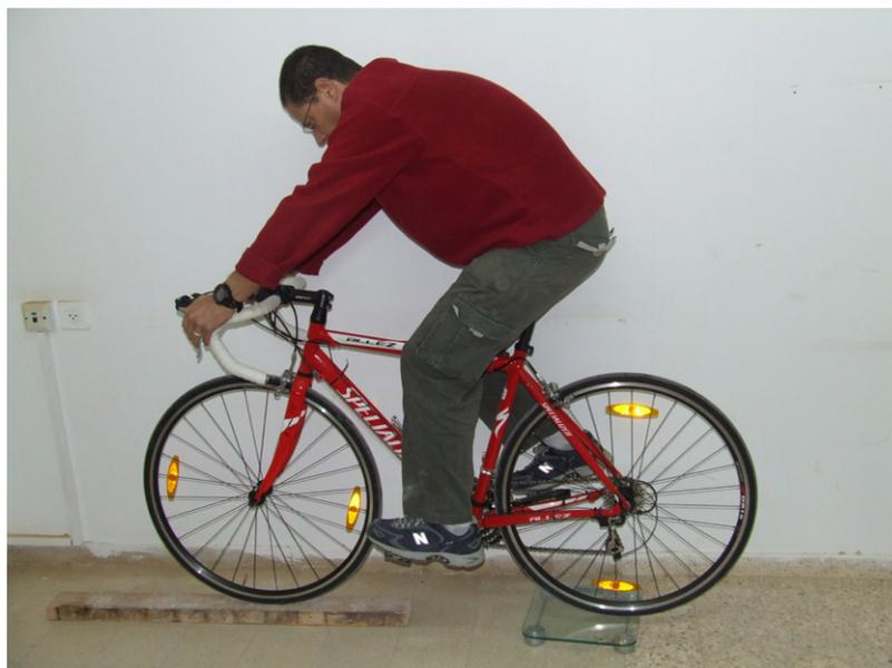
**Figure 1.** Measuring the normal force acting on the rear wheel of a road bike with a digital weight indicator. To help him stay balanced without support, for a brief time the rider has to use the wall and a person standing on the other side of the bike.
