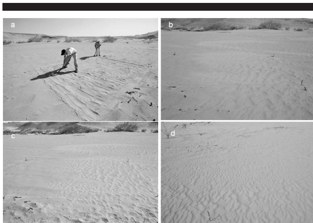
Figure 9. Preliminary results of field experiments done at Nahal Kasuy dune field in the Southern Negev, Israel. (a) The initial flattened plot (5 m × 5 m) of megaripples. (b) The plot after 62 d. There is no clear indication for the development of megaripples. The bed is covered with normal megaripples. (c) The bed after 75 d. (d) The bed after 102 d is covered only by normal ripples.
