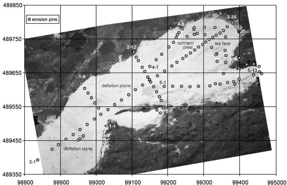
Fig. 3. Location of erosion pins and transects.
