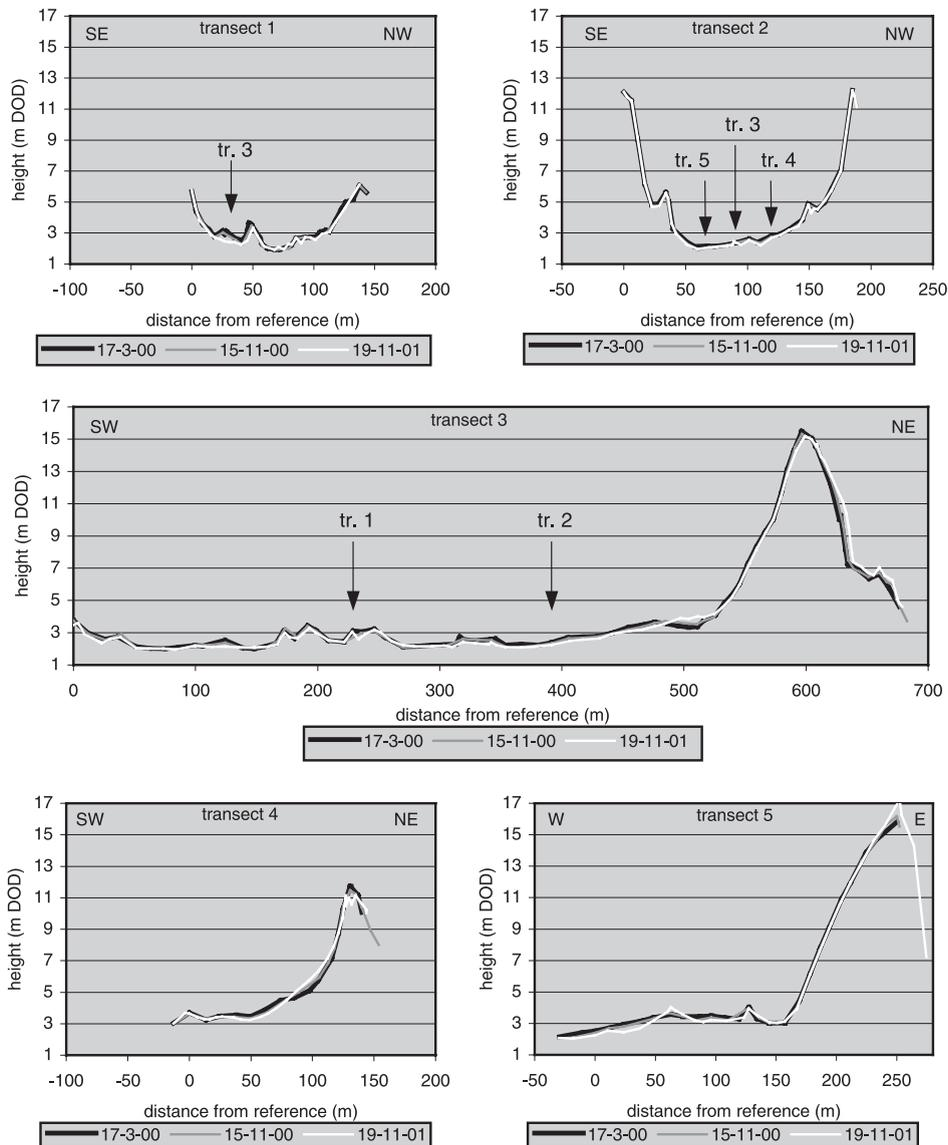
Fig. 6. Profile development of cross sections 1 to 5 between 17 March 2000 and 19 November 2001.
