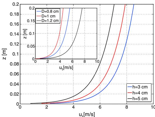
**Figure 4.** Threshold velocity for  $D_c = 1$  mm and  $u_* = 0.5$  m/s for ripples with different heights;  $z$  is the height above the surface. The inset shows the threshold velocity for different values of grain diameter (the other parameters are the same).
