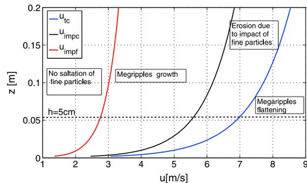
**Figure 5.** The different processes in megaripples evolution dictated by wind velocity at different height above the surface ( $z$ ). Parameters:  $h = 5$  cm,  $L = 0.2$  cm,  $D = 1$  mm, and  $u_* = 0.5$  m/s.
