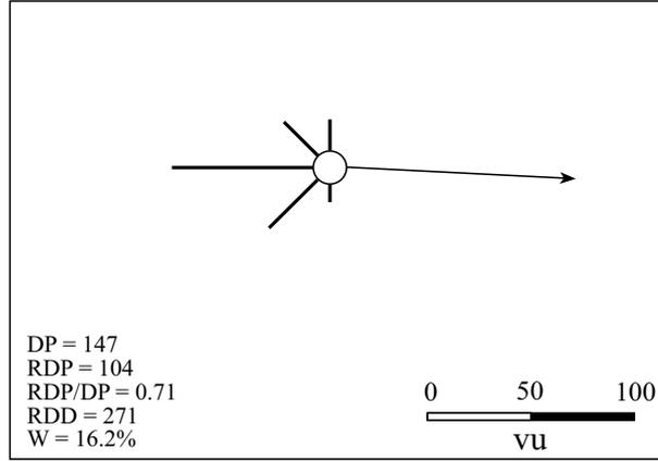
Fig. 1. Average annual sand rose for the coastal dunes south of Tel Aviv, Israel. The  $DP$  vectors are proportional in length to the potential sand transport in the direction toward the central point. The net potential trend of the  $DP$  vectors ( $RDP$ ) is shown by the arrow in the direction of the resultant drift direction ( $RDD$ ).
