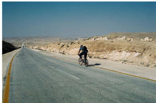
**Figure 3.** Carrying out the experiment on the declining road. The decline in the segment we chose is approximately constant and traffic there is very light. The best time to carry out this experiment is early in the morning in order to reduce wind effects on the experiment. The experimental distance should be at least half a kilometer.
