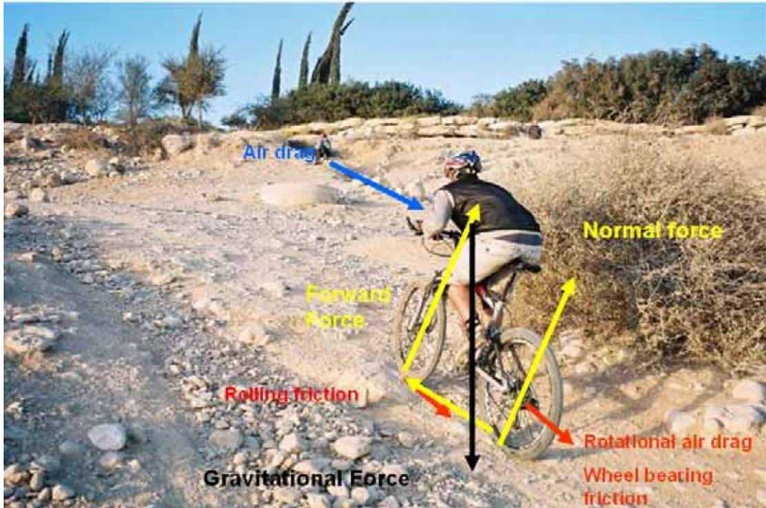
Fig. 1 The forces operating on a bicycle moving up an incline in a straight line. There are two main friction forces; the first is the rolling friction which dominates at low speeds while the air drag is dominates at high speeds.
