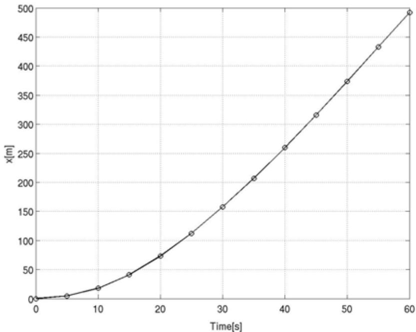
Fig. 6: The displacement as a function of time for the experiment described in Fig. 5. The displacement was calculated as the normal by integrating the velocity as measured by the Polar system.
