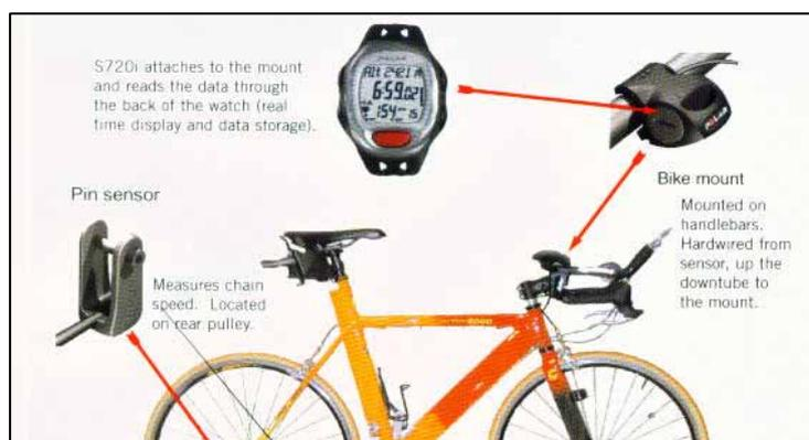
Fig. 3: Schematic diagram of the Polar S725X used to measure power exerted by the biker. The various factors are stored in a display unit attached to the bicycle and may be downloaded via an infrared device to a laptop computer. (Source: <http://www.polarusa.com/Products/consumer/s725x.asp>).
