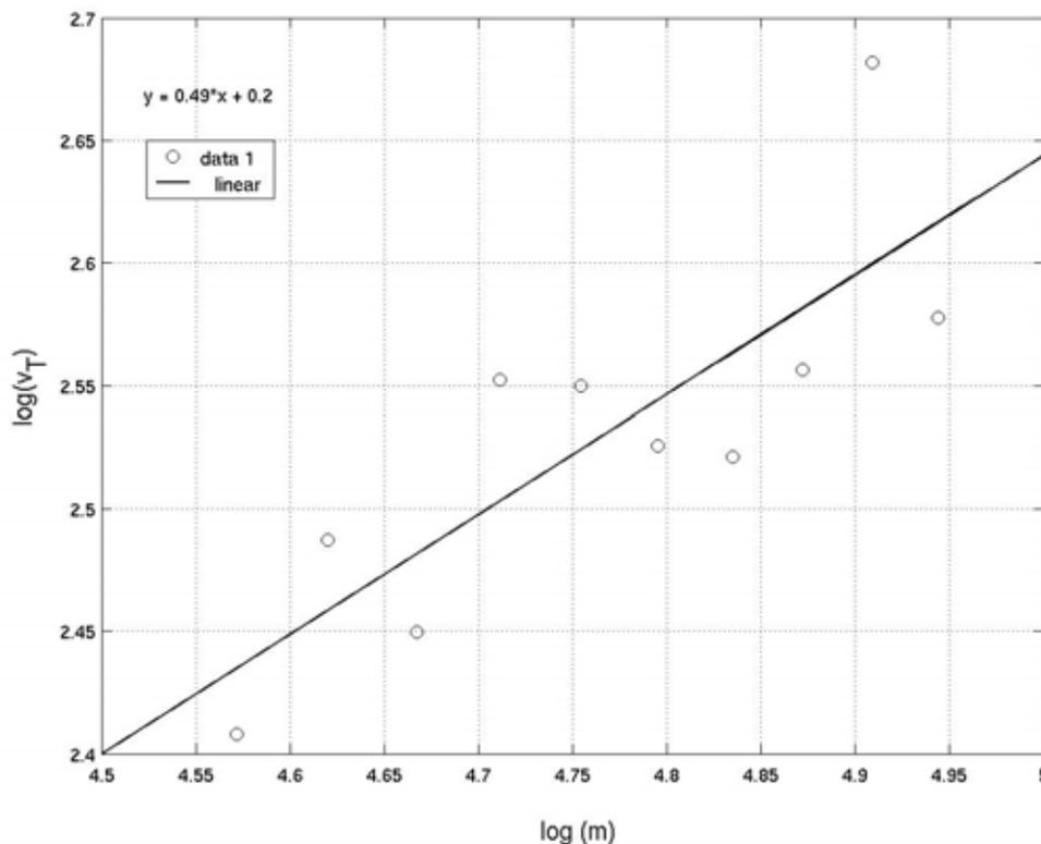
**Fig. 7:** Plot of  $\ln(v_t)$  as a function of  $\ln m$  for downhill experiment. The linear approximation of the slope is 0.49, extremely close to the theoretical slope of 0.5. The equation for the linear approximation is  $\ln(v_t) = 0.49 \ln m + 0.2$ .
