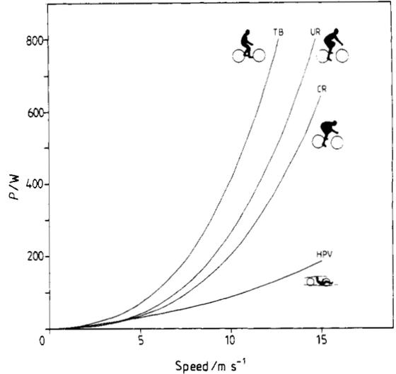
**Figure 3.** Power requirements for touring bicycle (TB), racing bicycle: upright (UR) and crouched position (CR), Vector vehicle (HPV).
