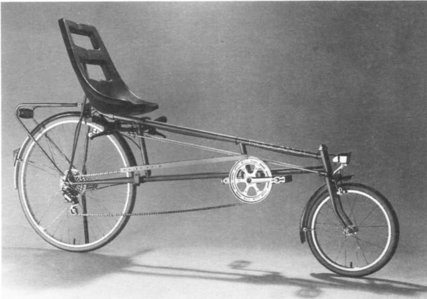
**Figure 4.** A reclining bicycle offers more comfort than a conventional bicycle. It can reach a speed comparable with that of a racing bicycle, but only on a level road.
