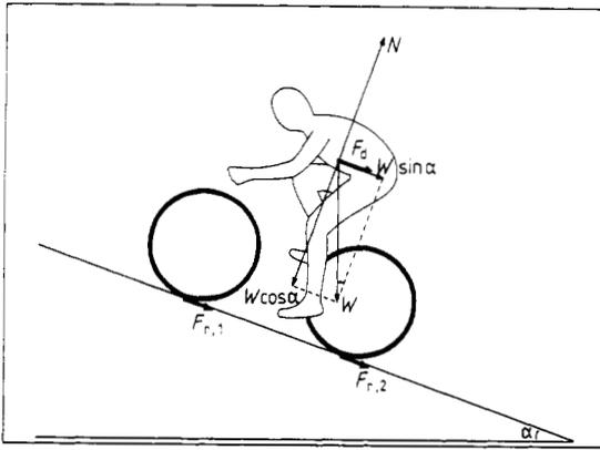
**Figure 1.** Rolling resistance  $F_r$  is proportional to the weight  $W$  of the vehicle due to gravity, and to the normal force  $N$  of the road on the vehicle.
