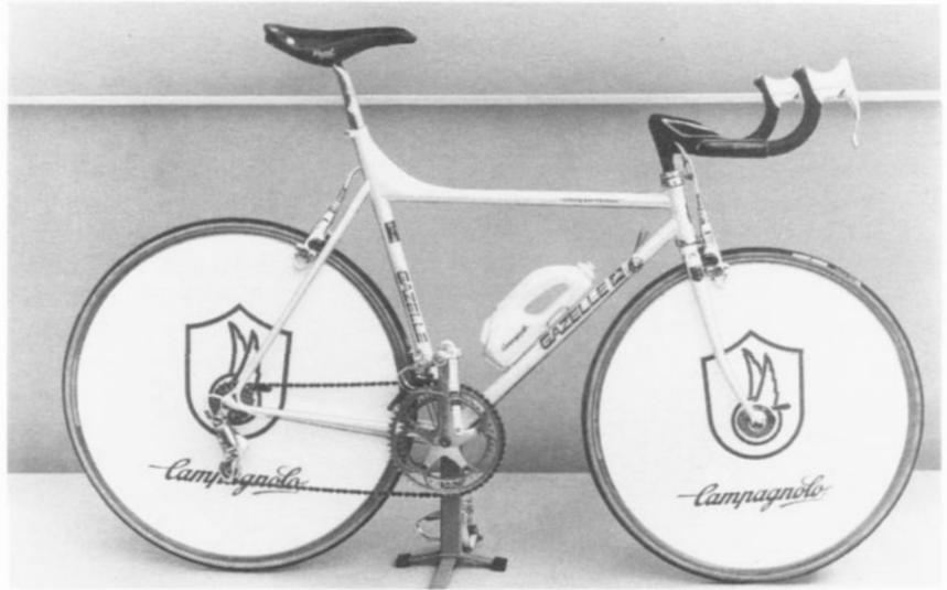
because its air drag is not significantly less than that of the conventional racing bike, the reclining bicycle never attained a real breakthrough. (A well designed recumbent can be faster by 3 or 4% than the racing bike, at 75 W.) Racing bicycles are often even faster, especially in hilly landscape, when the weight of the vehicle becomes important and the advantage of streamlining disappears.
