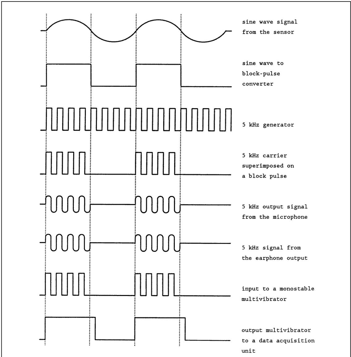
Figure 4. Transformation of the original sine wave signal.
