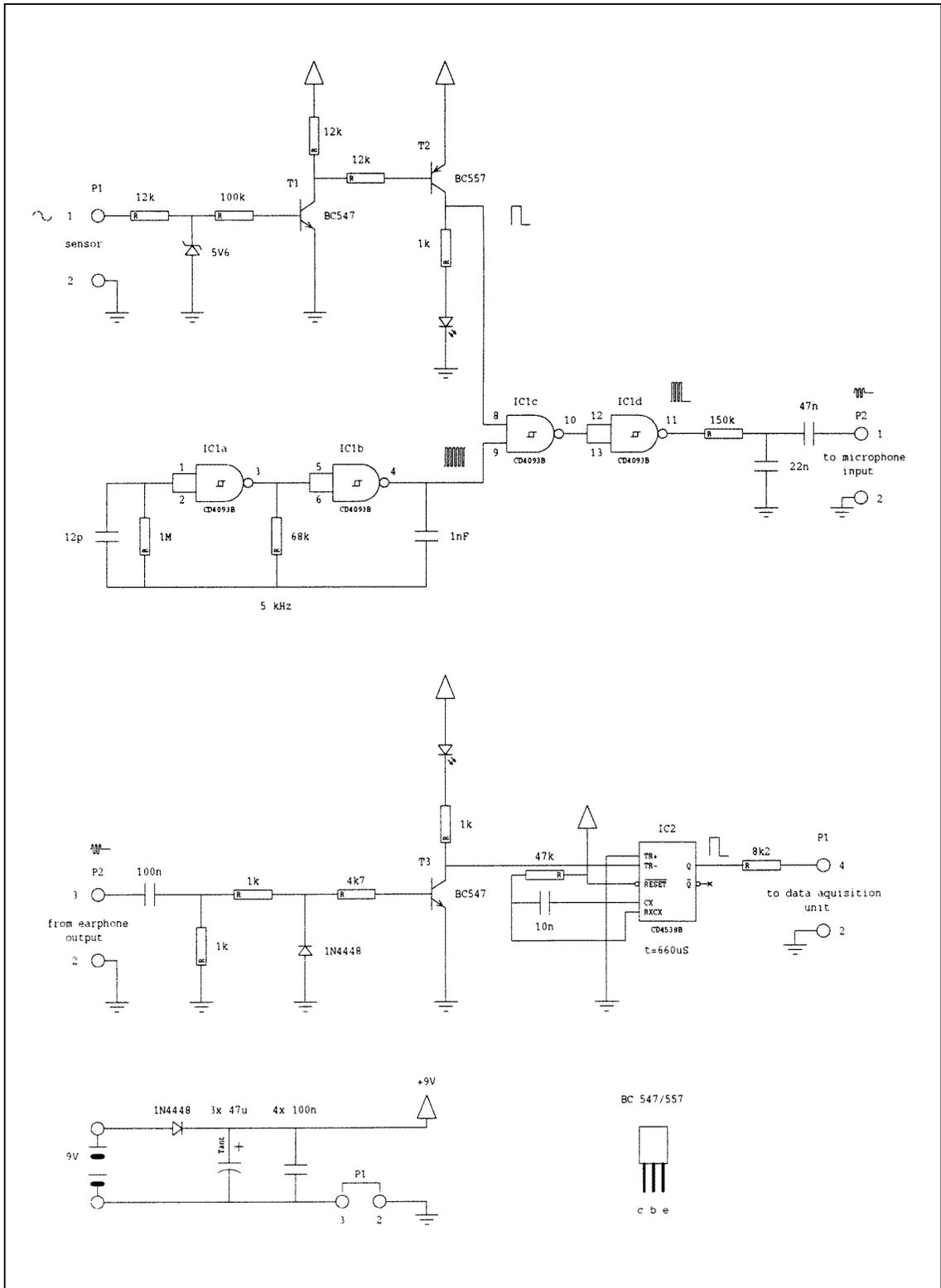
Figure 5. The wiring of the SC.
