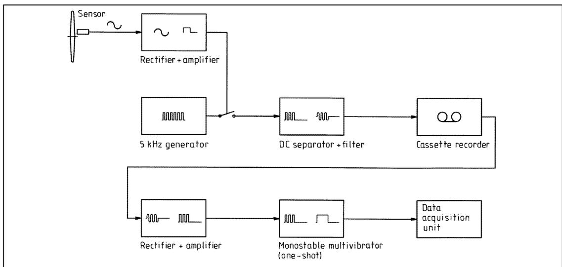
**Figure 3.** Block diagram of the signal converter (SC).
