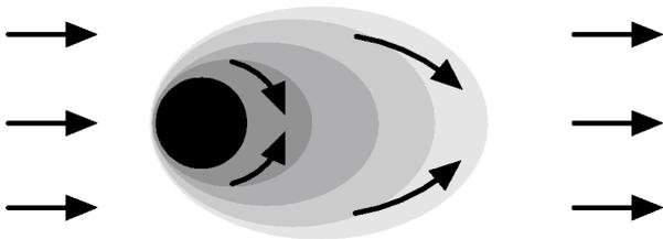
FIG. 2. Wind direction and speed around a plant. The normal wind speed area is white; absence of wind inside the plant is indicated by black; transition areas are shades of gray. Wind directions are indicated by arrows. While this only crudely approximates real flows, it captures the essence of the flow pattern around a plant.
