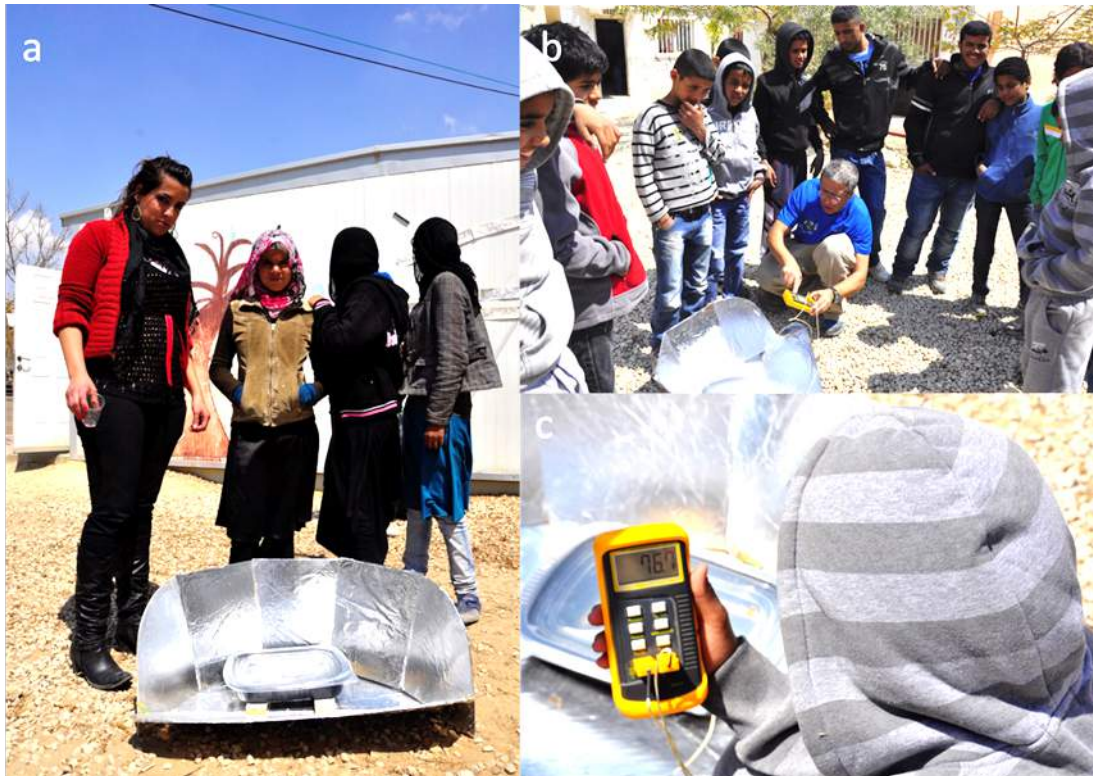
Fig. 8. (a) A group of three girls and their science teacher with the finished solar cooker; (b) Employing a digital thermometer to show the Bedouin students the temperature that can be reached in the panel cooker; (c) a student measuring air temperature inside a plastic baking pan (suitable for high temperatures) in the panel cooker.
