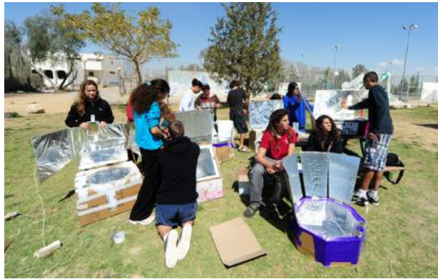
Fig. 5. Stagnation tests for box cookers (left) and test results for the 6 groups (right). Ambient temperature during this time was 20 C.
