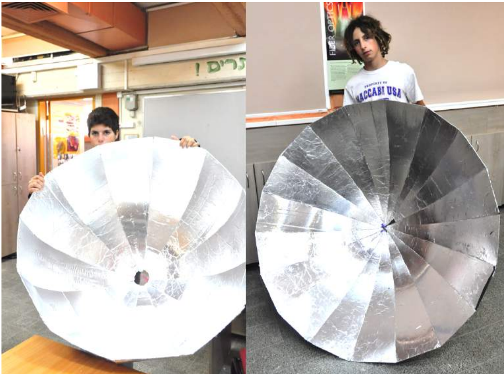
Fig. 4. The assembled concentrators; left the hemisphere – right a paraboloid.
